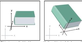
Object axes (in black) move with the object; global axes (in gray) are fixed.
