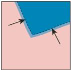
Spread (object overlaps background) compared to choke (background overlaps object)
